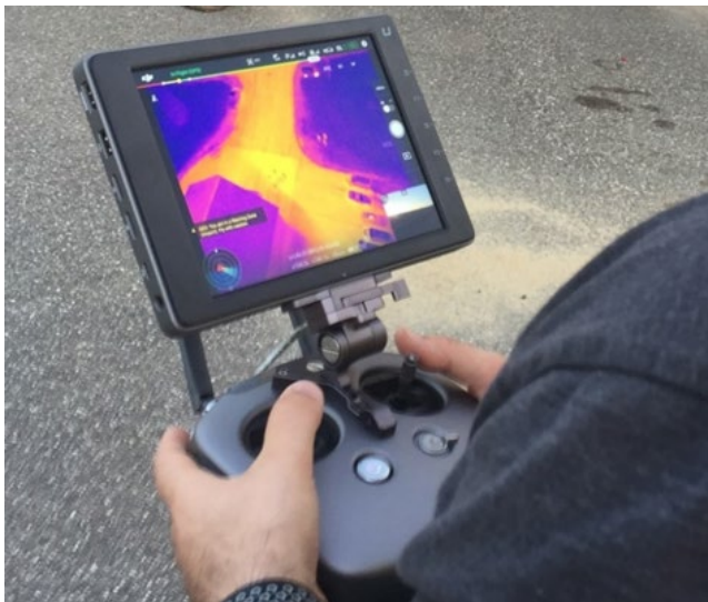
Figure 6 – DJI flight controller using the Zenmuse FLIR XT camera
