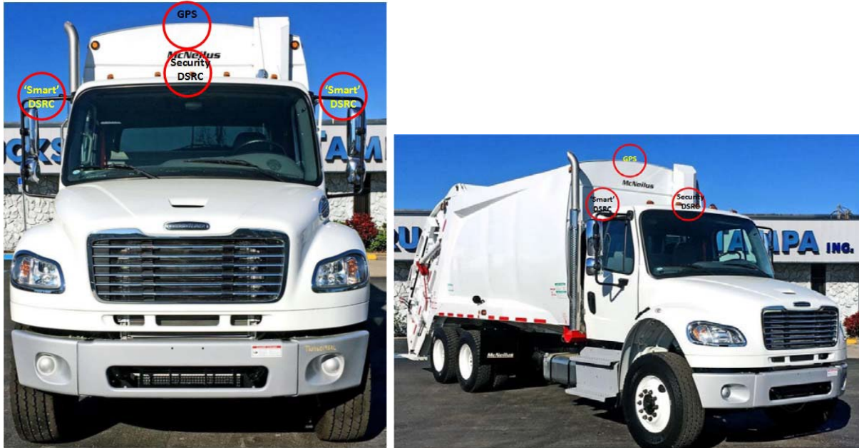
Figure 13: Retrofit Configuration 3 for use with specific truck tractors, straight trucks, buses, and vocational trucks
