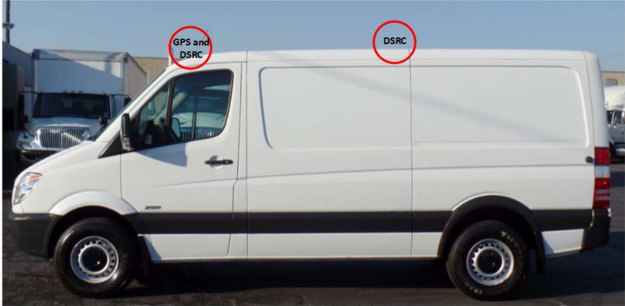
Figure 11: Retrofit Configuration 1 for buses, motor homes, and most straight trucks Configuration 2, shown in Figure 12, is a fairing mounted design that applies to nearly all truck tractors with articulated trailers that use fairings.
