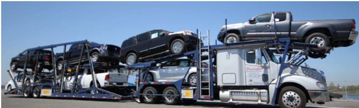
Figure 10: Difficult or expensive vehicles to retrofit due to an absence of a viable location for the GNSS antenna
