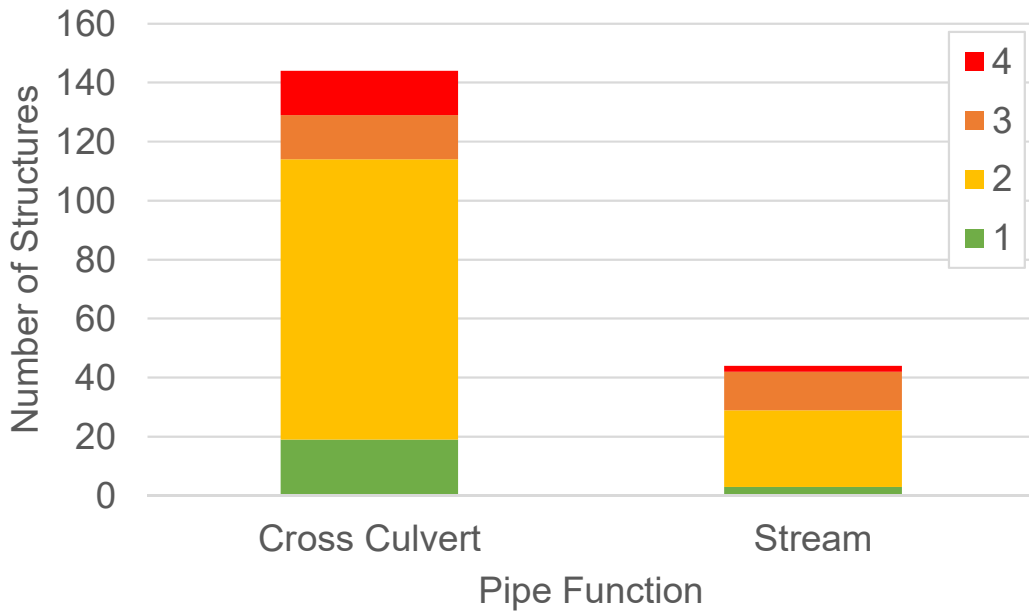
Figure C.17 Histogram of reported pipe function with reported corrosion rating.
