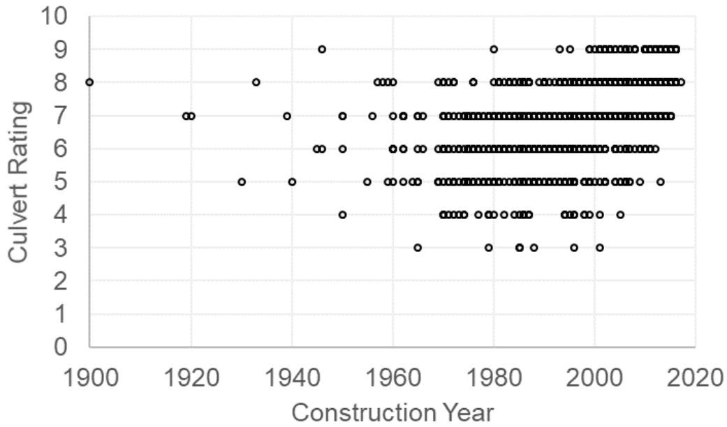
Figure C.26 Culvert rating vs. construction year.
