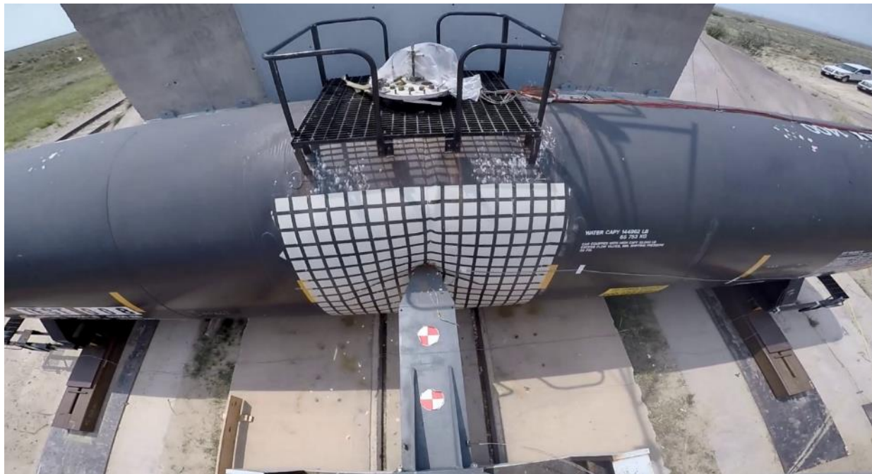
Figure 14. Deformed Tank Just Prior to Puncture
