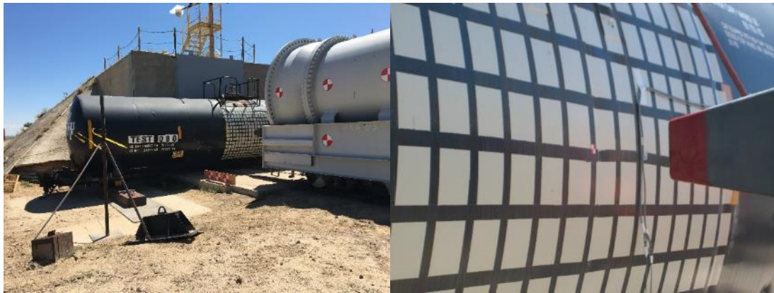
Figure 8. Overall Test Setup (left) and Ram Arm with 6-inch by 6-inch Indenter Aligned with Center of the Tank Car (right)
