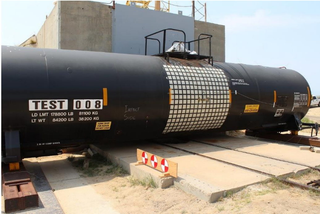
Figure 4. Target Tank Mounted on Support Skids
