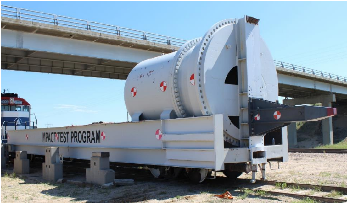
Figure 6. Ram Car and Head (i.e., from a previous test with 6-inch by 6-inch indenter)
