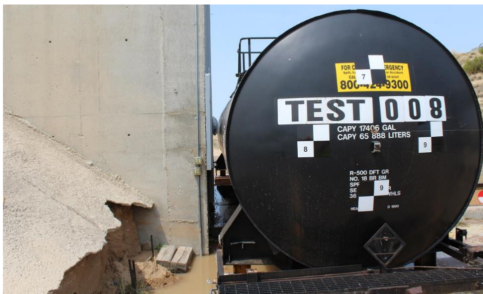
Figure 16. Tank Car—Post Impact (wall side)
