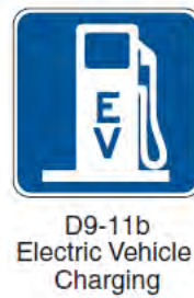
Figure 23: Electric vehicle charging sign as defined in FHWA's MUTCD
