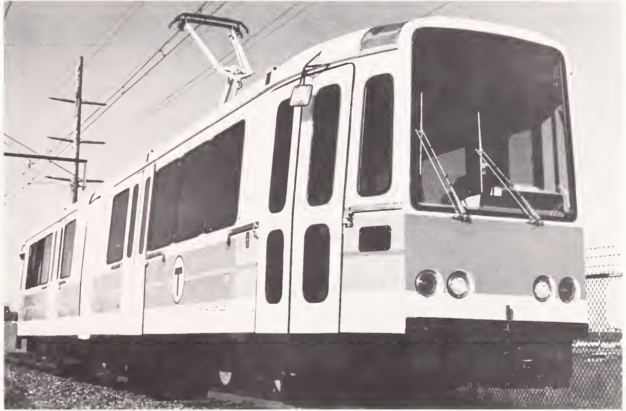
The New Standard Light Rail Vehicle is in Service in Boston and San Francisco.
