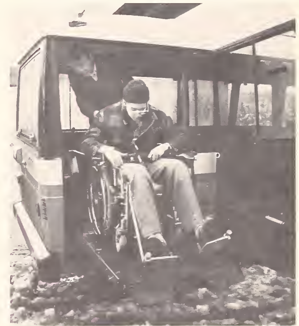
Portland, Oregon's LIFT Program Features Demand-Responsive Buses Equipped with Wheelchair Lifts.
