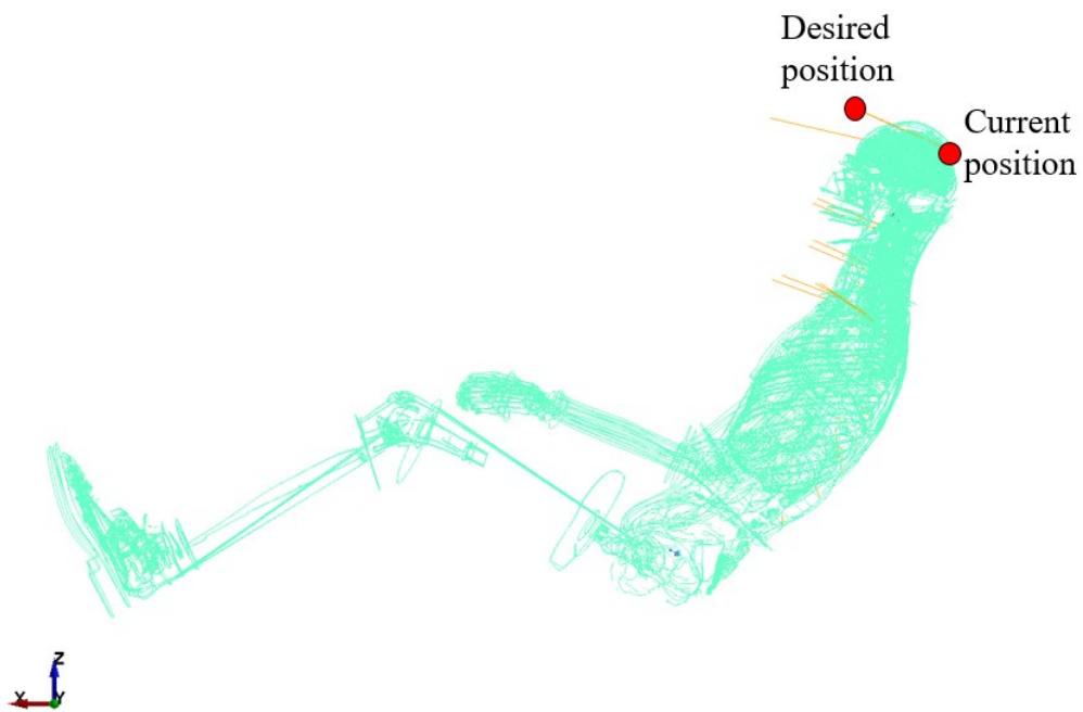
Figure 43. Cable pulling method for the M50-O upper body to match positions in the M50-OS.
