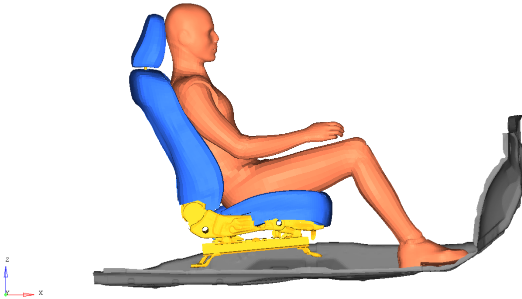
Figure 30. Upright (25°) seated M50-OS in the final position after lowering the arms.
