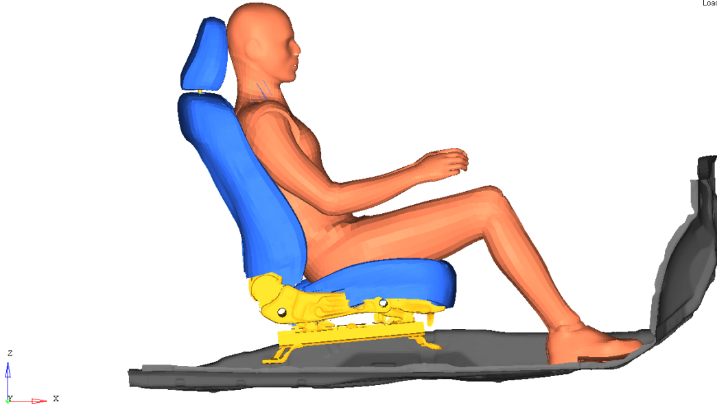
Figure 25. Upright (25°) seated M50-OS after gravity settling only.
