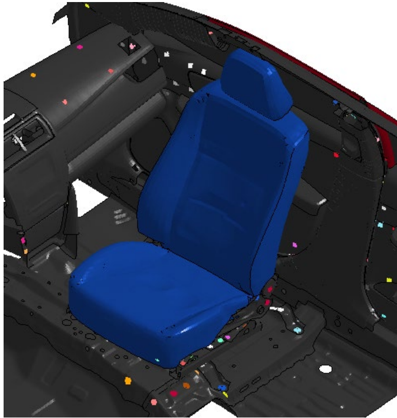
Figure 7. Passenger seat in the 90-degree orientation after positioning.
