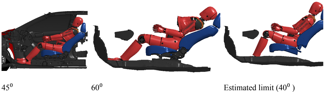
Figure 22. THOR FE model integration into reclined seat.
