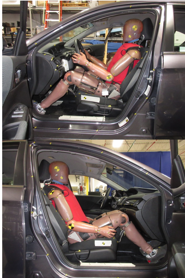
Figure 2. THOR: (a) Driver Seat; (b) Passenger Seat.
