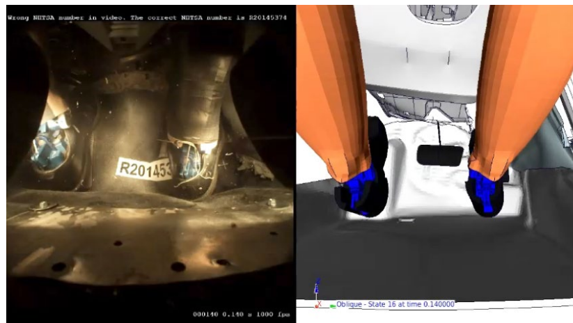
Figure 4. Lower Leg Kinematics in Test and Simulation.
