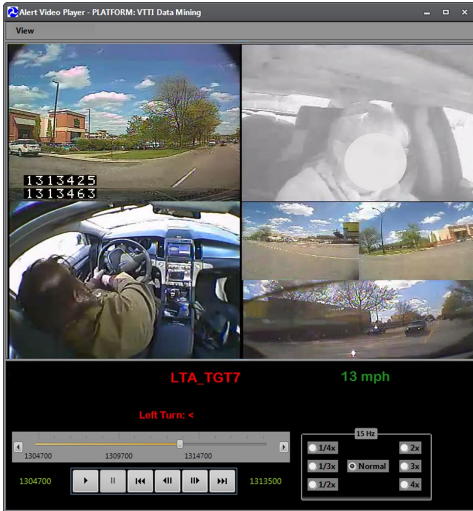
Figure 12. Screen Capture of Tool for Reviewing Onboard Camera Videos
