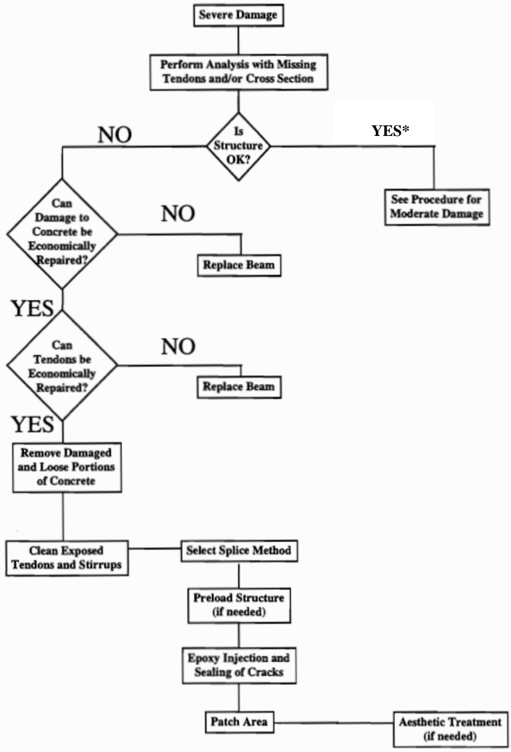
Figure 2.3. Flowchart for repair of severely damaged girders (from Feldman et al., 1996) (*apparent typographical error has been corrected).
