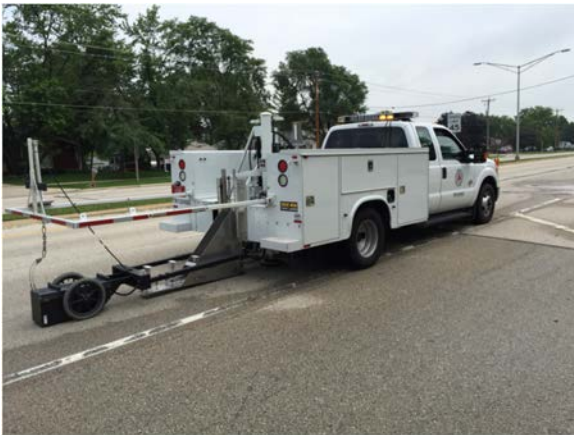
(a) FWD testing on STH 100 in Oak Creek
