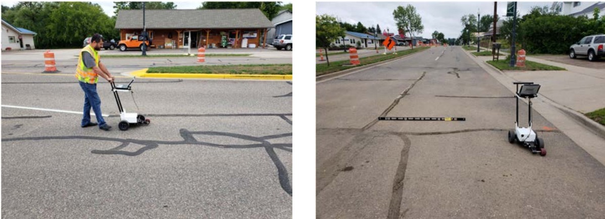
Figure 3.3: The CS8800 Walking Profiler System provided by Surface Systems & Instruments, Inc. used to measure pavement surface profiles.
