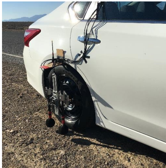
Figure 15. Example of OBSI microphone array mounted on a passenger car (VOLPE CENTER)
