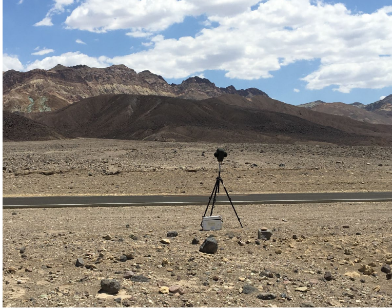
Figure 17. Example of binaural recording, binaural head setup at S03 (VOLPE CENTER)
