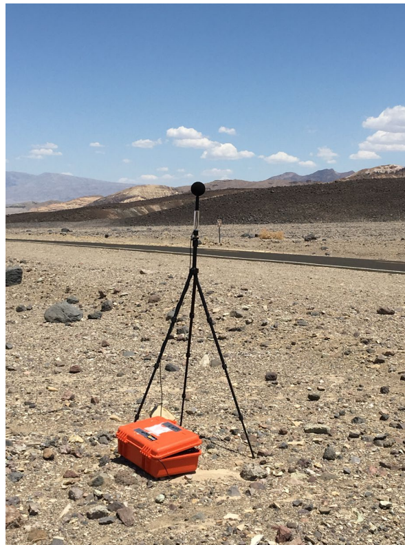
Figure 16. Example wayside measurement setup at site S03 (VOLPE CENTER)
