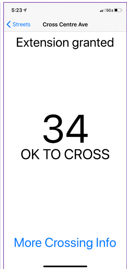
Figure 10: A screenshot of the PedPal app informing the user that an extension was granted, it is ok to cross, and there are 34s remaining in the crossing phase for Centre Ave.
