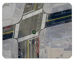
Figure 2d: Through bicycle and vehicle right turn lane, through intersection guidelines, no mixing zone, bicycle signal and phase separation/concrete median separation from right turning vehicles.
