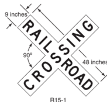
Figure 1. Illustration. A crossbuck as depicted in the Manual for Uniform Traffic Control Devices .
