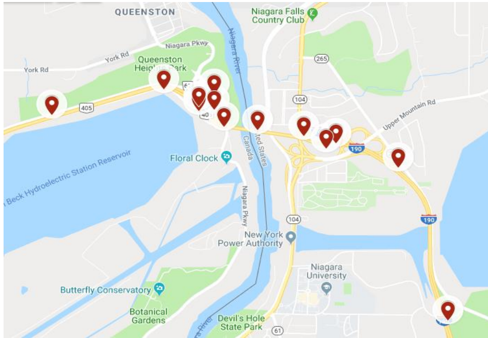
Figure 24. Location of Bluetooth readers at Queenston Lewiston Bridge
