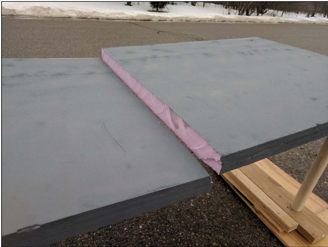
Figure 48. Photo. The model bridge with a raised section used to represent bridge settlement for the UAS data collection.
