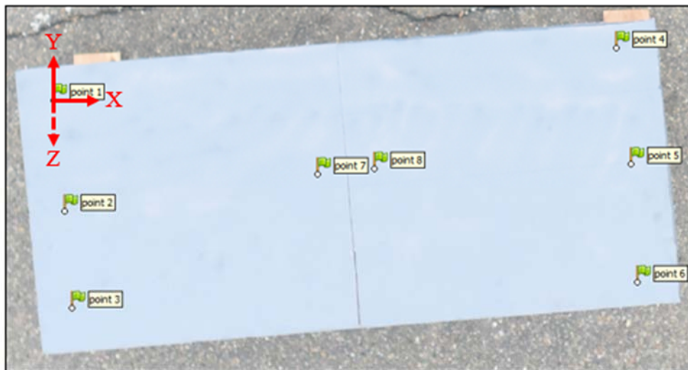
Figure 47. Illustration. Picture of model bridge with position of coordinate markers 1-6. Additional markers 7 and 8 used for reporting Z-axis position.
