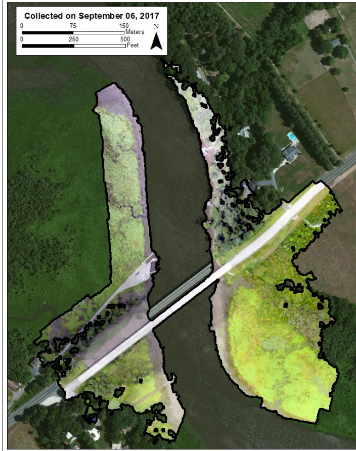
Figure 28. Illustration. DJI Phantom 3A aerial imagery (outlined in black) reconstructed into an orthophoto image with 3D elevation data shown on top of an GIS Basemap displaying WorldView satellite imagery (Tuckahoe Creek).
