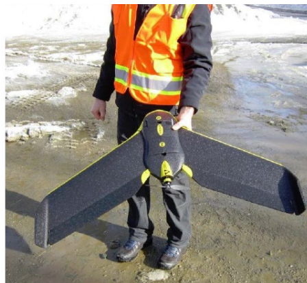
Figure 5. Photo. A fixed wing UAV used to collect CRS data.
