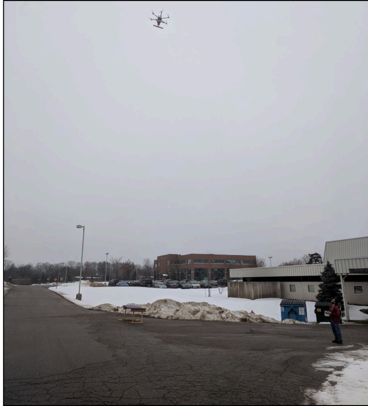
Figure 49. Photo. Certified remote pilot collecting imagery from the UAS of the model bridge in the settlement scenario.
