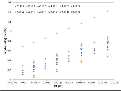
Fig. 5. Logarithmic plot of the viscosity (mm<sup>2</sup>/s) in function of 1/T [K<sup>-1</sup>].
