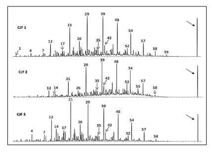
Fig. 2. GC/MS chromatograph of Commercial Jet Fuels.
