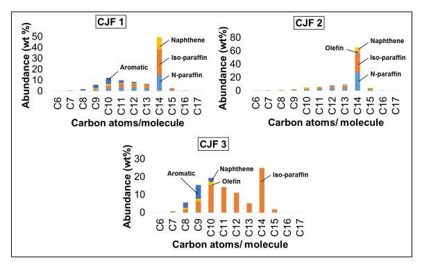
**Fig. 4.** Weight percentage of each class of hydrocarbons identified in the commercial jet fuels by GC-MS
