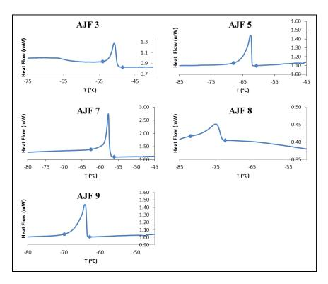
**Fig. 6.** DSC results for the alternative jet fuel samples. The base ("shoulder") of the peaks, indicated by diamond mark, represents the measured cloud point temperatures. Fuels AJF 1, AJF 2, AJF 4 and AJF 6 did not show any peaks within the range of temperature used in this analysis.
