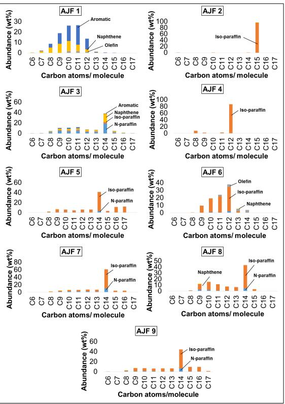
**Fig. 3.** Weight percentage of each class of hydrocarbons identified in the alternative jet fuels by GC-MS
