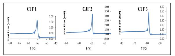
**Fig. 7.** DSC results for commercial jet fuel samples. The base ("shoulder") of the peaks, indicated by diamond mark, represents the measured cloud point temperatures. The pour point estimation is indicated by a circle mark.
