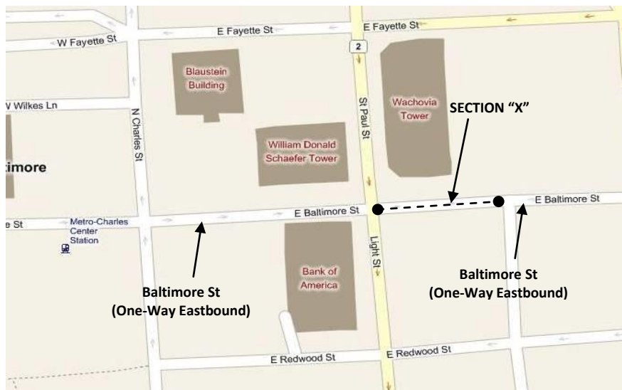
Figure 4.4: One-Way Roadway (Code '1') Example
