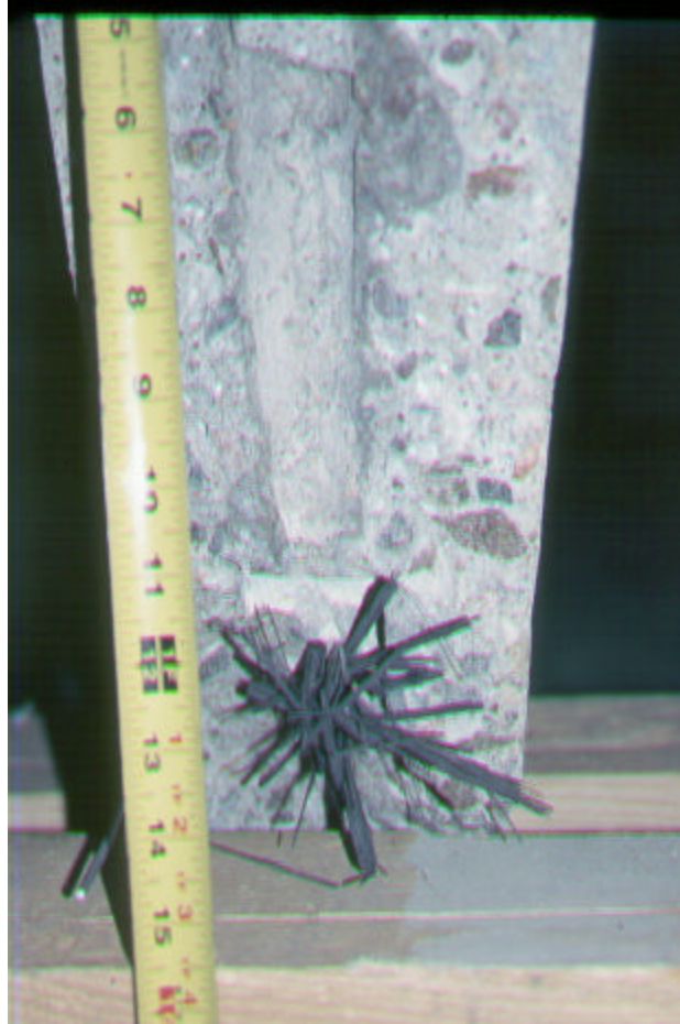
Figure 13.3 Carbon Tendons After Failure
