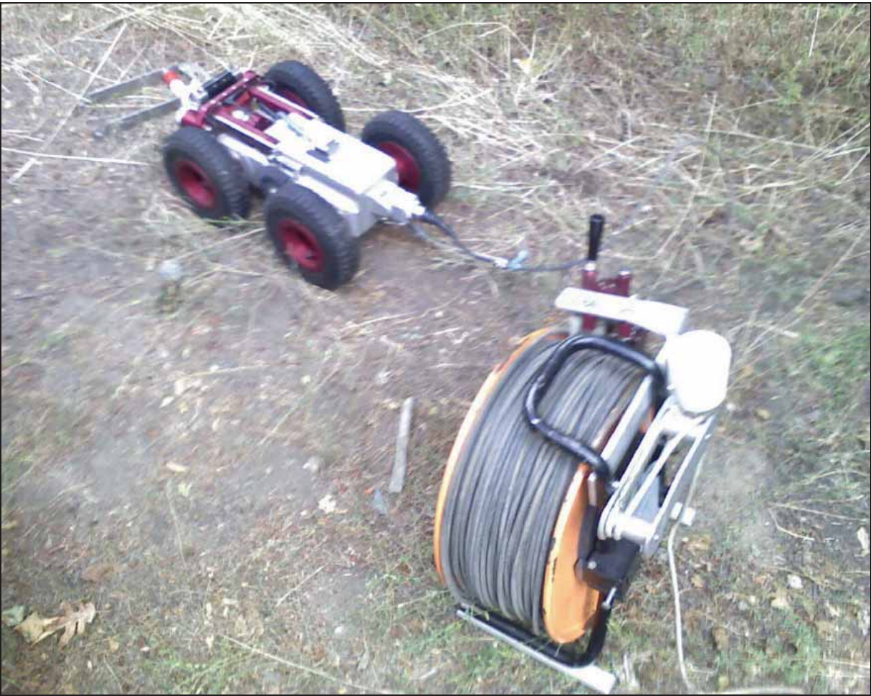
Figure 48. Photo. Pipe crawler ROV system ready for Level 2 inspection of CMP example in Yosemite National Park.
