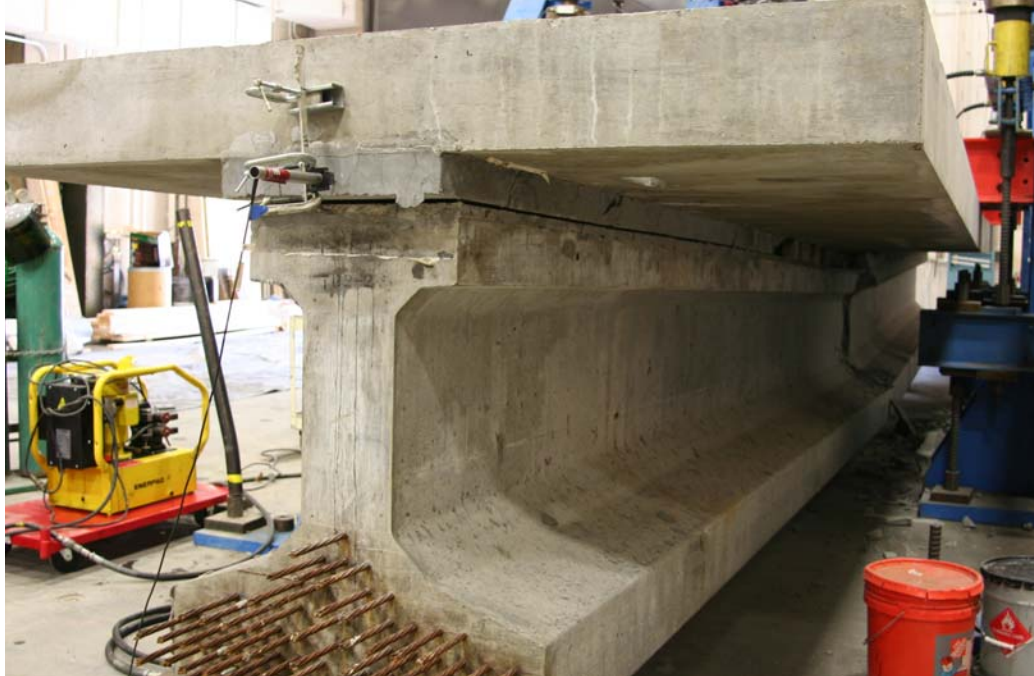
Figure 51. Photo. East end and north face of test specimen immediately after completion of test.
