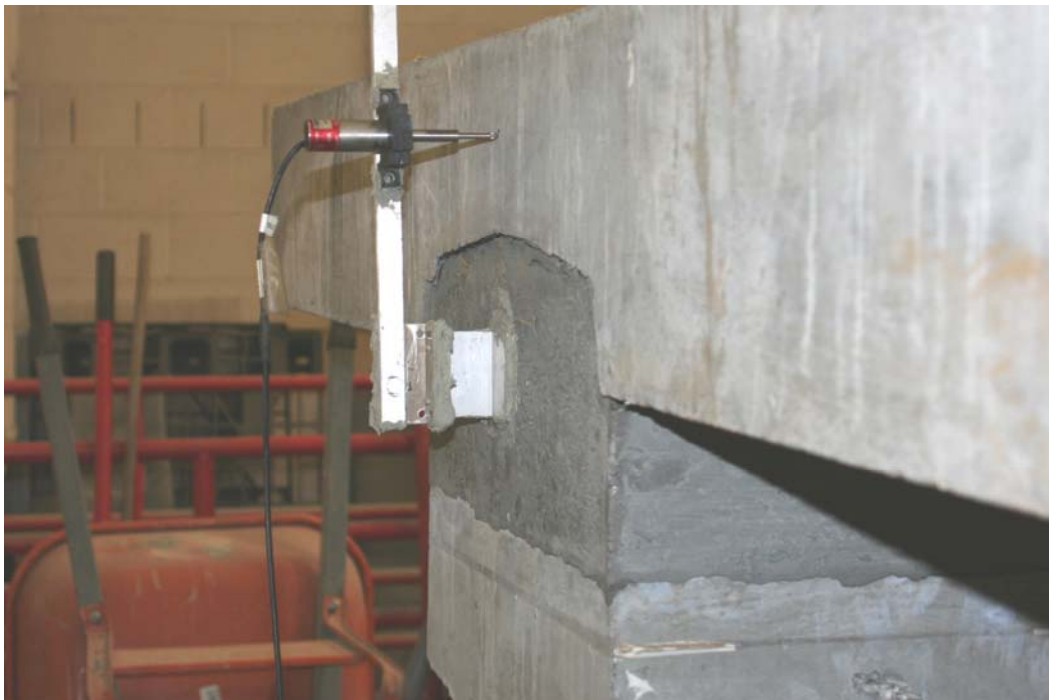
Figure 29. Photo. Haunch connection which emulated the composite connection to a concrete girder (i.e., west end) immediately before the attainment of peak applied load.
