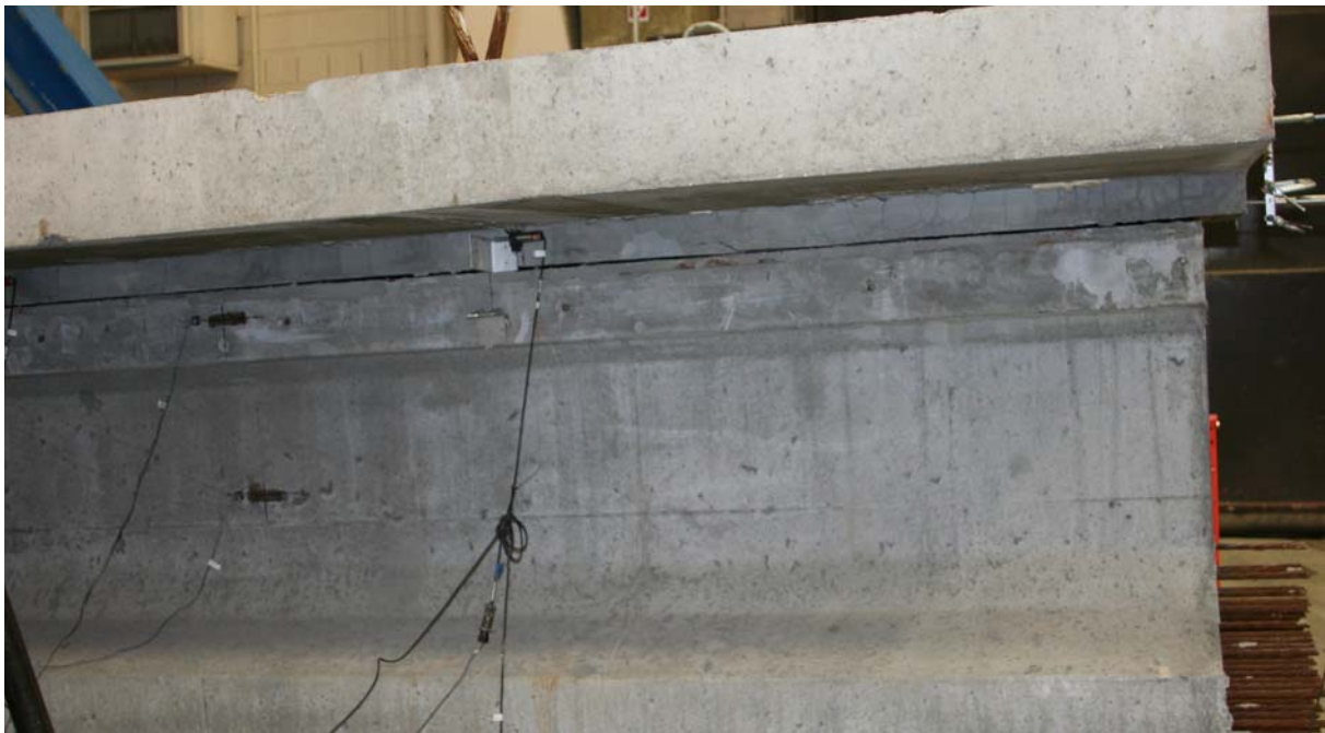
Figure 50. Photo. Haunch connection on south face at east end of test specimen immediately after completion of test.
