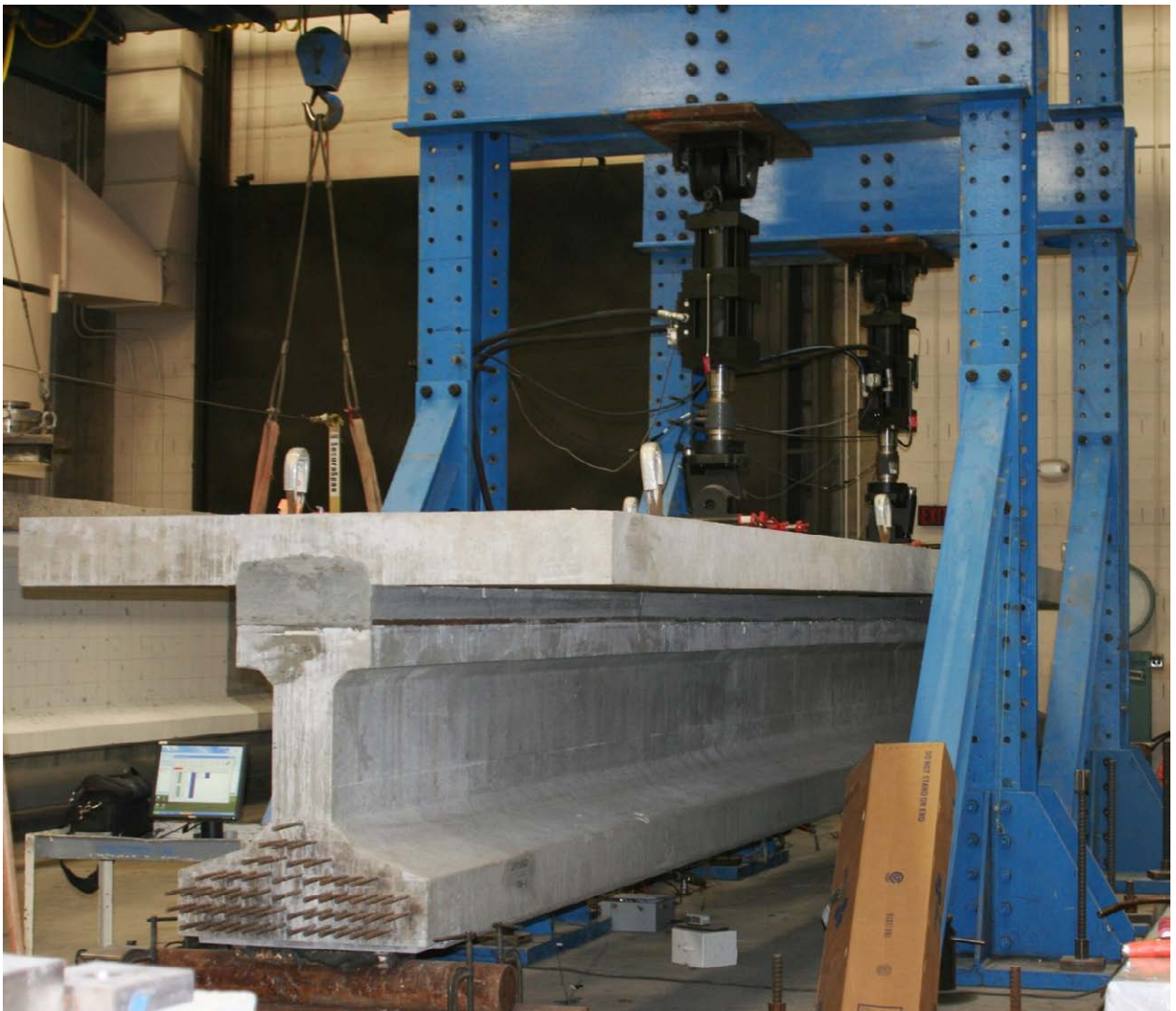
Figure 13. Photograph. Overall test setup for cyclic test program.
