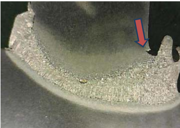
Fig. A11. Sample S-1. Asymmetrical, but adequate weld. Note ductile failure initiation near the stud HAZ, arrow, representing the preferred mode of failure for cases wherein the stud welds has good quality.
