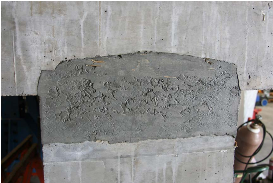
Figure 23. Photo. Haunch connection at portion of test specimen which emulated the composite connection to concrete girder (i.e., west end) at conclusion of cyclic testing.
