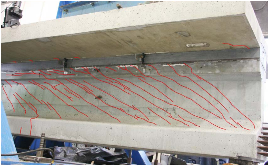
Figure 33. Illustration. Cracking apparent on south face of east end of test specimen after completion of static testing.
