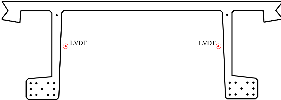
Figure 42. Illustration. Lines C and E LVDT locations for Tests P4-57Sh and P4-57Ss.
