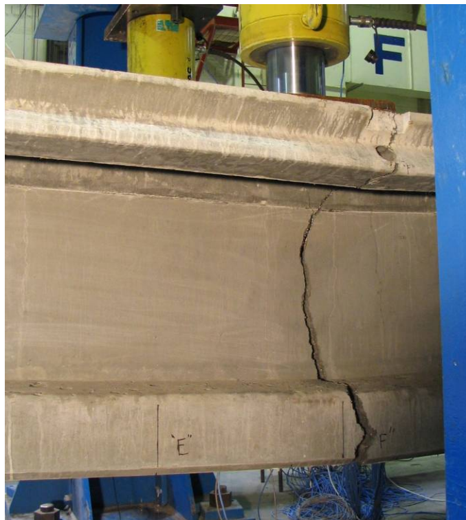
Figure 135. Photo. Flexural failure of P4-57Ss south leg.
