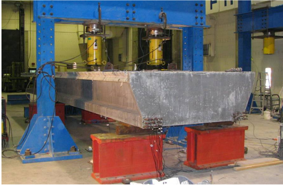
Figure 25. Photo. Setup for second load configuration of Test P2-21S.
