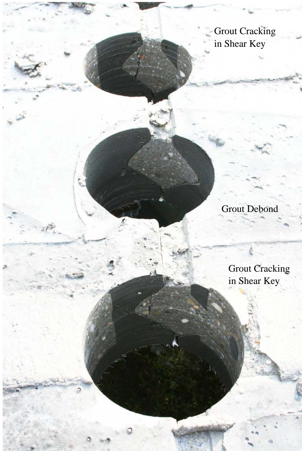
Figure 85. Photo. Distress visible inside core holes after Test T2J.
