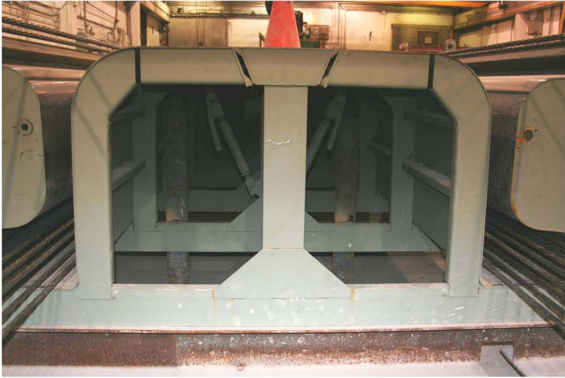
Figure 9. Photo. Girder formwork.
