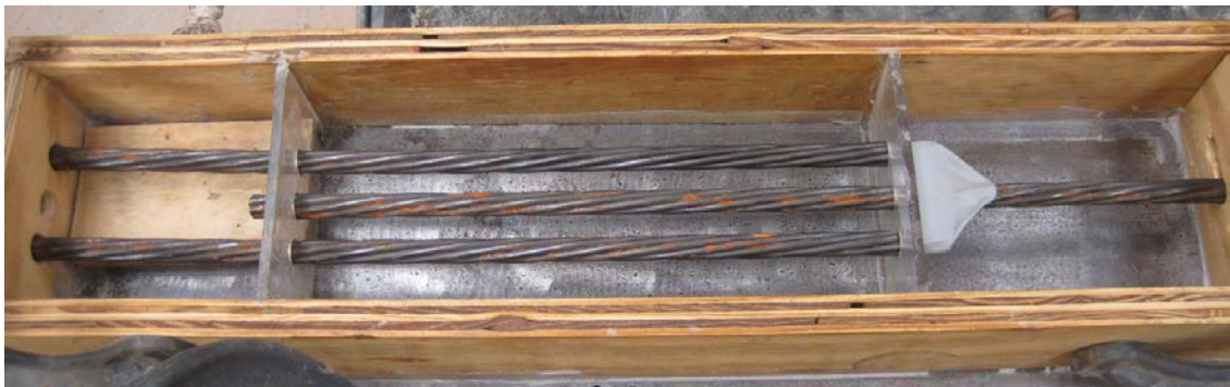
Figure 2. Photo. Form with strands for 12 inch (30.5 cm) long test specimen.
