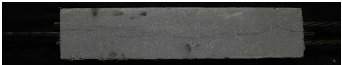
Figure 14. Photographs. Cracking apparent at conclusion of testing of R2D specimens.
