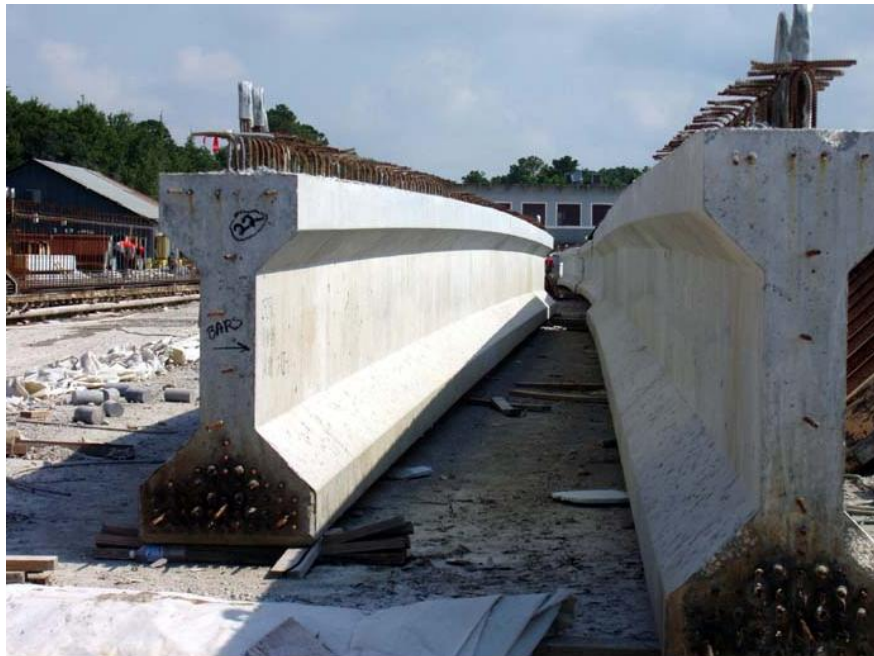
Figure 2.37 Residual, upward deflection from prestress and self-weight
