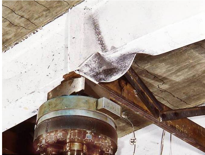
Figure 2.20 Local Buckling of Compression Flange
