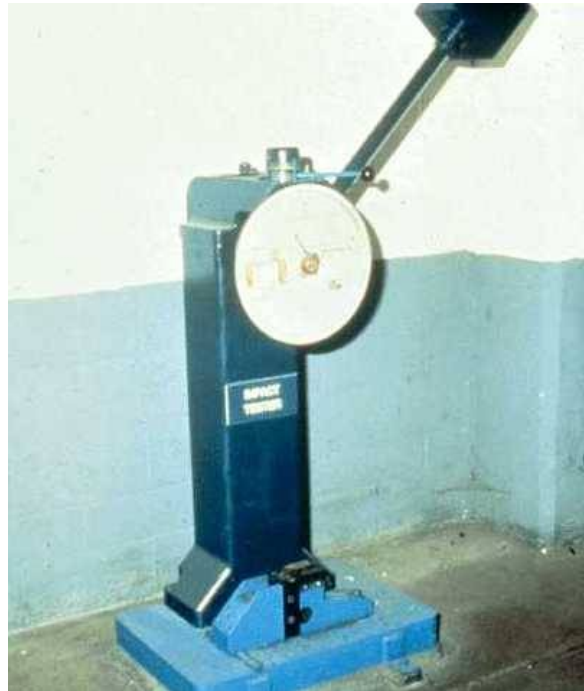
Figure 2.56 Charpy V Notch Testing Machine
