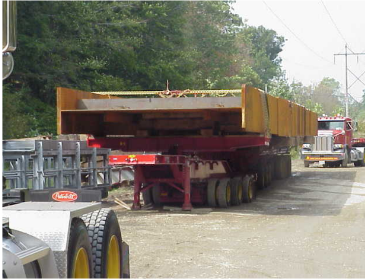
Figure 2.26 Bridge Girder Transported on Side
