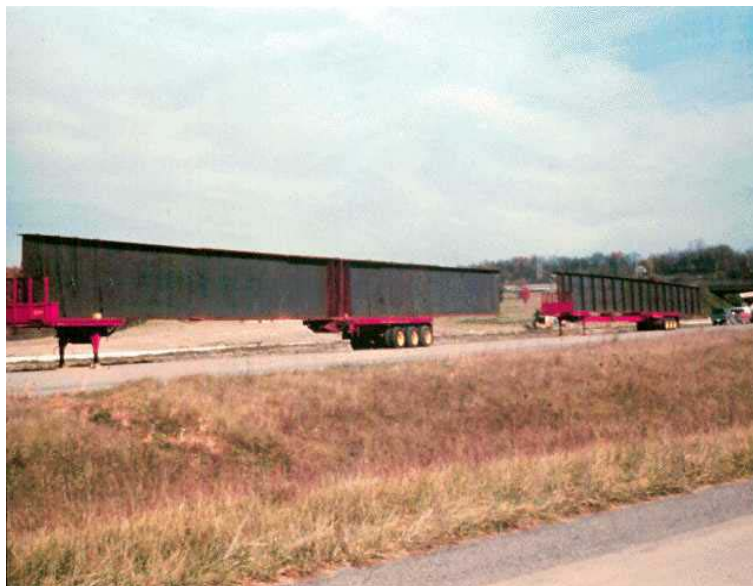
Figure 2.25 Transporting Bridge Girders by Truck
