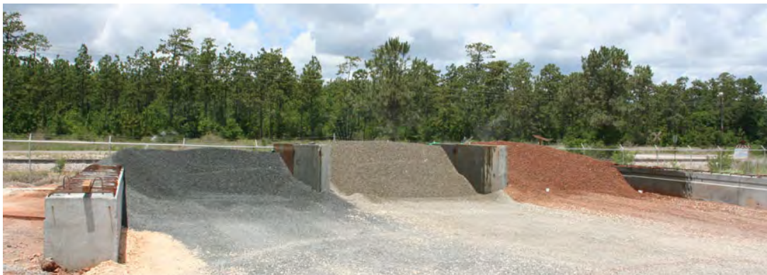
Figure 6. Photo. Lightweight Aggregate Stockpiles at Precaster's Facility with Continuous Sprinklers.
