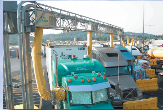
A simple window adapter makes this electrification system compatible with many models of long-haul trucks. Photograph courtesy of IdleAir.
