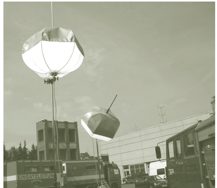
Figure 14. Powermoon lighting system.
