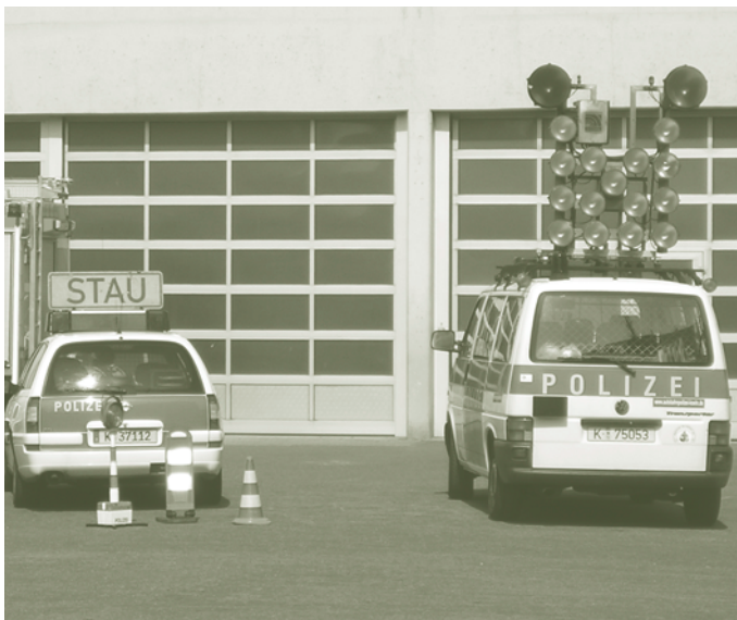
Figure 9. German end-of-queue warning vehicles.
