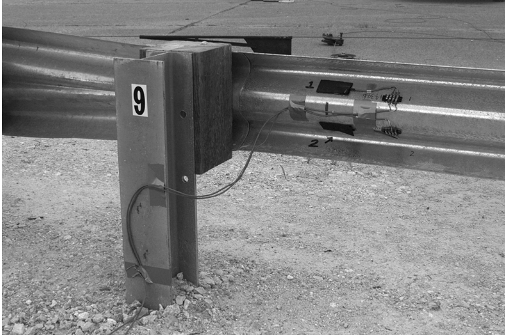
a) Strain gauges on W-beam rail element.
