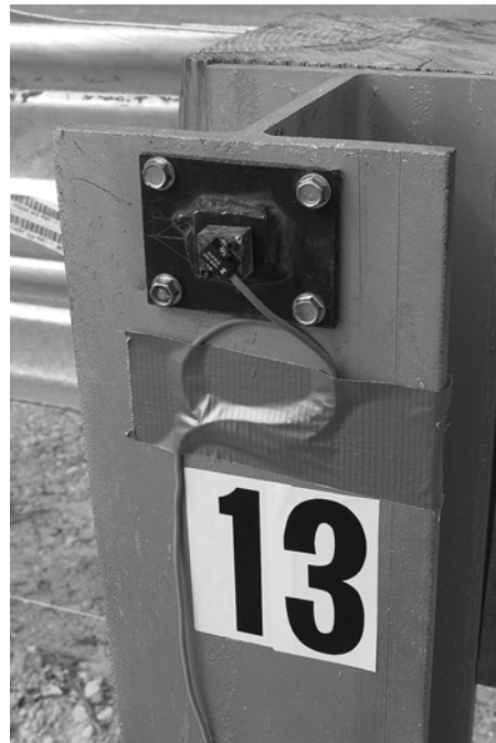
b) Accelerometer on post 13.
