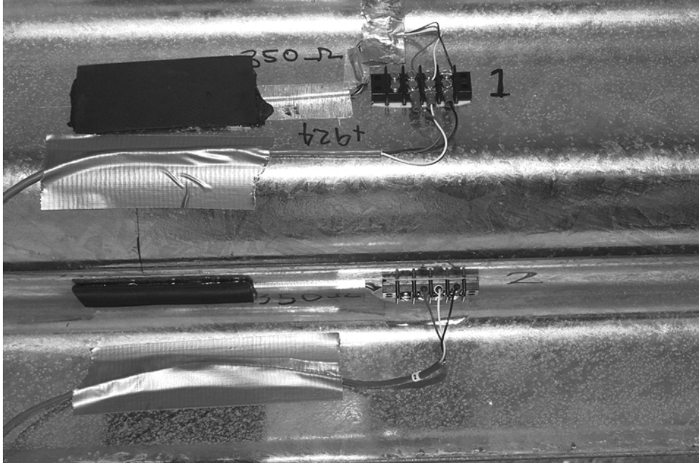
a) Strain gauges on rail.
