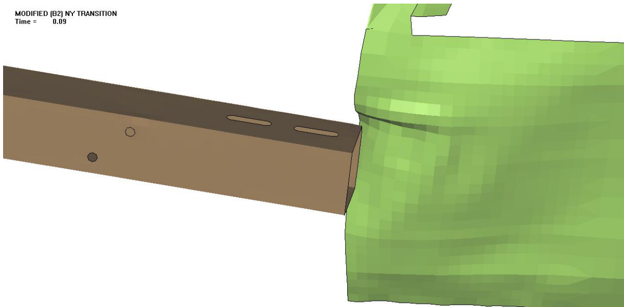
Figure 71. Door edge contact with the rail splice.
