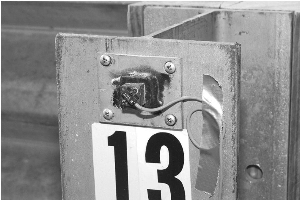
b) Accelerometer on post 13.
