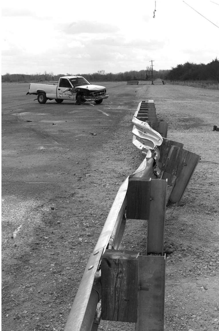
Figure 15. Vehicle trajectory path after test 401021-6.
