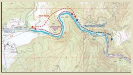
Figure 4.2D – The proposed road location was surveyed on the ground by specialists in soils and botany. The survey identified old disturbances that had revegetated naturally over the last 50 years to a community of native grasses and forbs. Several disturbed reference sites (RR1, RR5 and RR6) were identified. Intensive soil and vegetation surveys were conducted at each site. For the new stretch of forest road, undisturbed reference sites (UR2 and UR4) were identified and surveyed.
