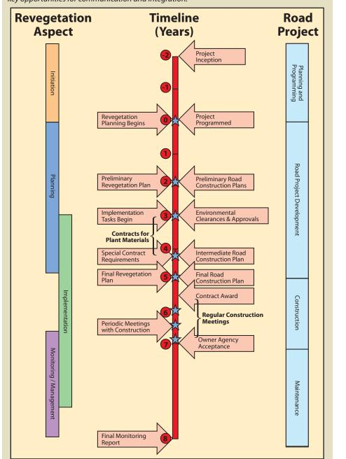
**Figure 2.1** – Coordinating revegetation with the larger processes of road construction is essential. While the timelines and agencies involved will vary, this figure illustrates some of the key opportunities for communication and integration.
