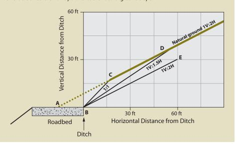
for soil erosion is considerably reduced. Furthermore, there is a substantial cost savings with less excavation and revegetation work. Figure 5.51 gives an example of how increasing the steepness of a cut slope on a typical 1V:2H natural ground slope substantially decreases the length of disturbed soils.
