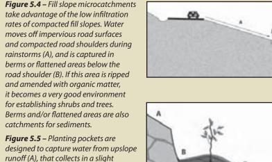
designed to capture water from upslope runoff (A), that collects in a slight depression (B). Captured water wets up the soil after each rainstorm and drains into the fractured bedrock (C). Soil is protected from surface erosion on the downhill side of the pocket with mulch or erosion fabric (D).
