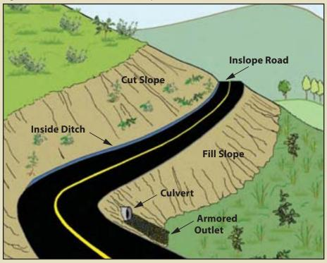
Figure 3.9 – Terms used to describe road slopes.
