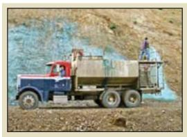
**Figure 10.97** – The hydraulic seeder is composed of a tank that holds and mixes a slurry, and a pump system that moves the slurry through a nozzle for application to the soil surface.
