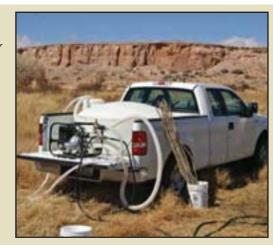
**Figure 10.111** – A 250-gallon water tank with pump can be installed in the bed of a pickup truck to supply water for Waterjet Stinger sticking. Introduction
