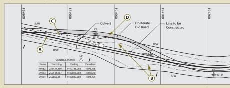
line), bottom of the fill slopes (Figure 3.1 C, dashed lines), and the location of the original road (Figure 3.1 D, shaded area). In this example, the original road will be obliterated.
