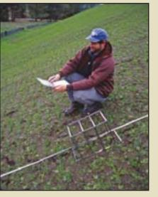
**Figure 12.3** – A fixed frame can be adapted to allow for the positioning of a laser pointer at 20 points in the frame. Soil cover or plant cover attributes are recorded at each laser point. The frame in this example is 8 in by 20 in, with 2 in spacing within rows and 4 in spacing between rows. The laser is a Class Illa red laser diode module that produces a 1mm dot.
