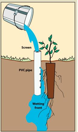
compacted, the amount of water that is delivered to the lower rooting zone can be reduced. A better method of water delivery to the root zone of trees and shrubs is to bypass the surface of the soil completely.
