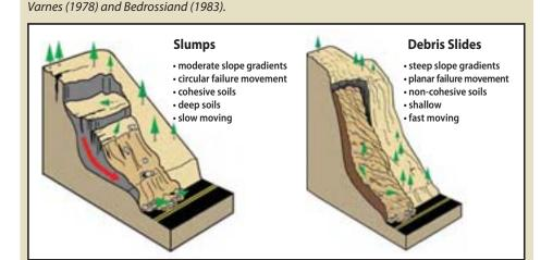
Figure 5.55 – Common landslides typically associated with road construction. Modified after
