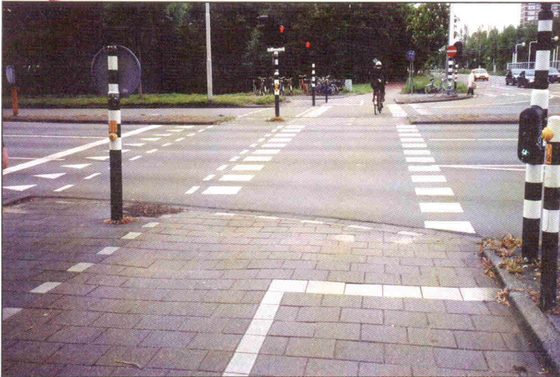
Figure 4-18. Nearside bicycle signals in the Netherlands.
