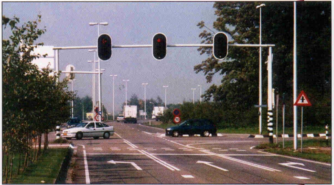
Figure 4-11. Large back-plate bordered by white stripe.
