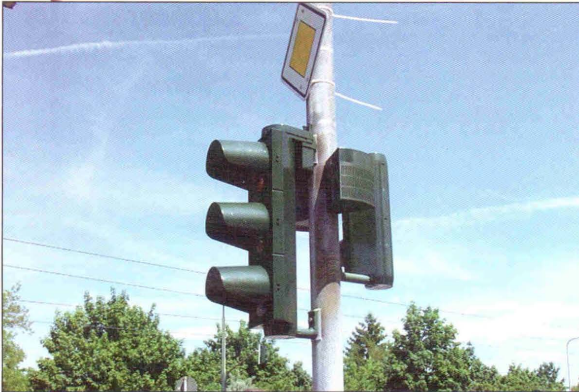
Figure 4-8. Pole-mounted audible signal in Germany.
