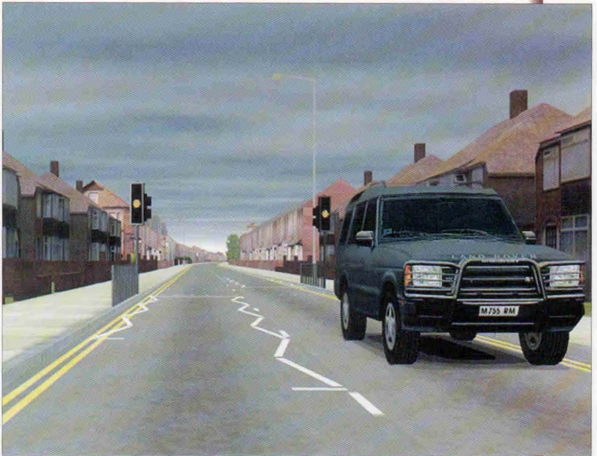
Figure 2-5. Vehicle simulator to test extended amber timing in the United Kingdom.
