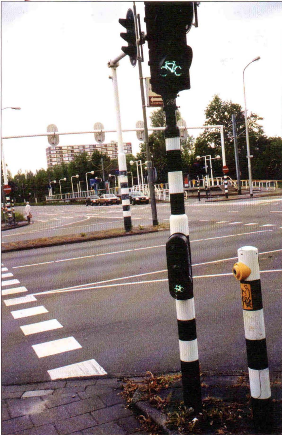
Figure 4-10. Signal poles with high-contrast stripes.
