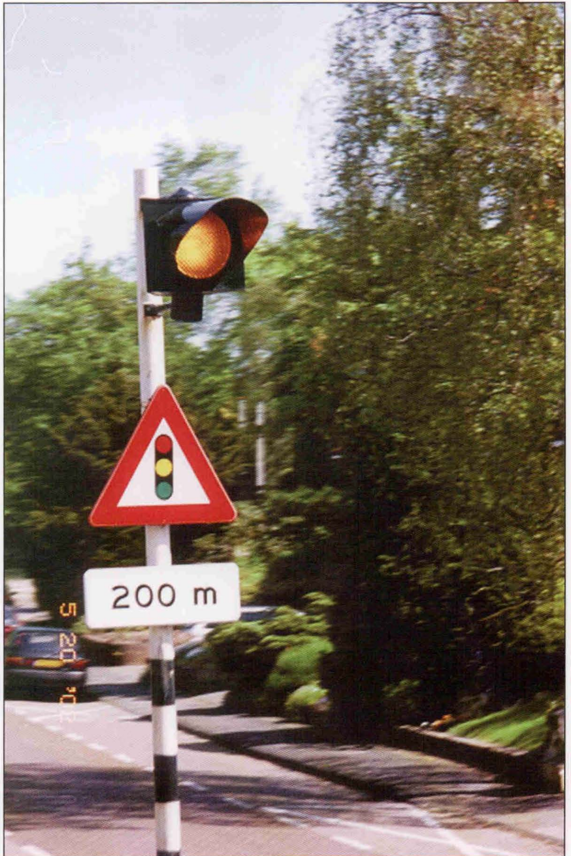
Figure 4-9. "Signal ahead" warning sign in the Netherlands.
