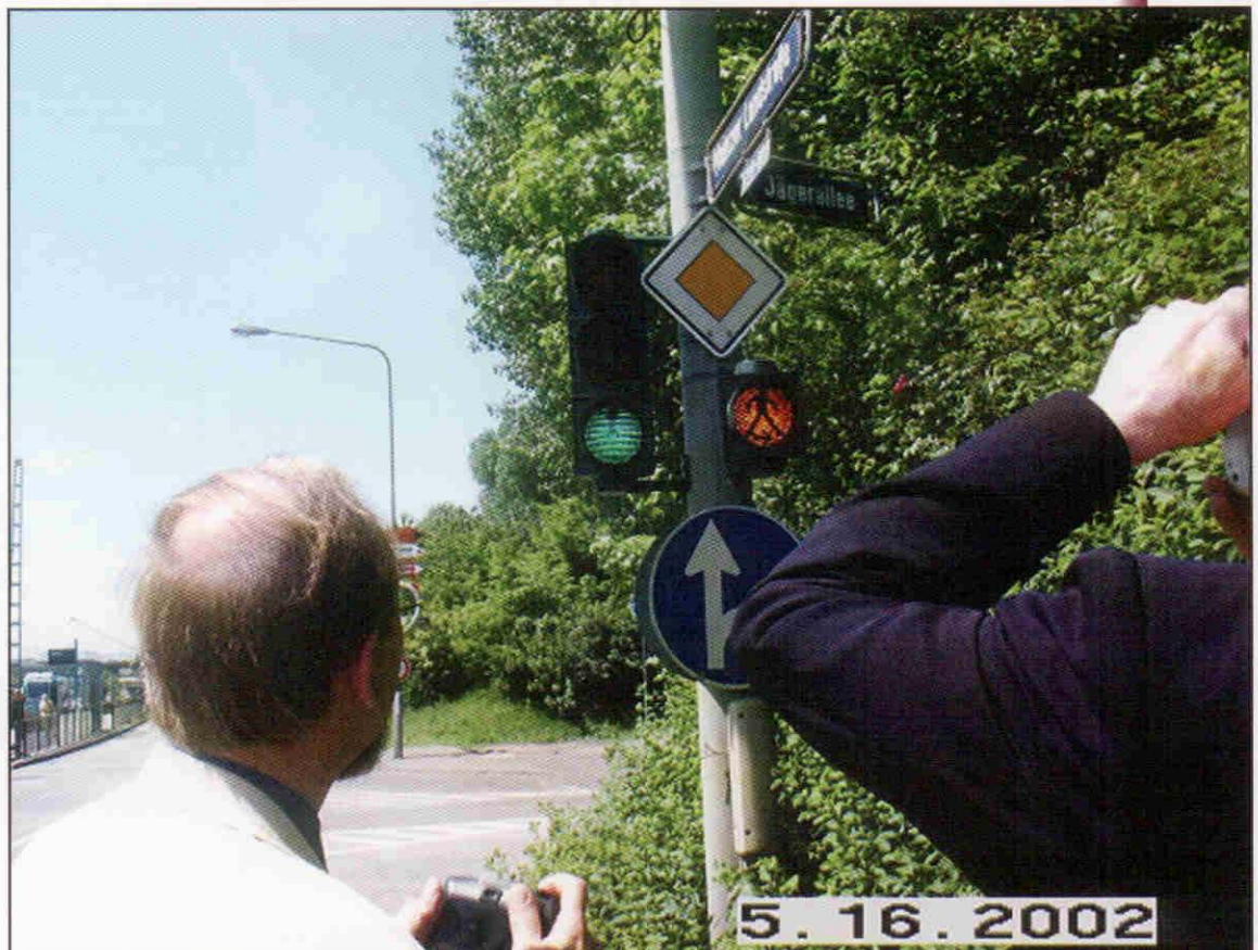
Figure 4-7. Supplemental signal warning right-turning motorists about pedestrians.
