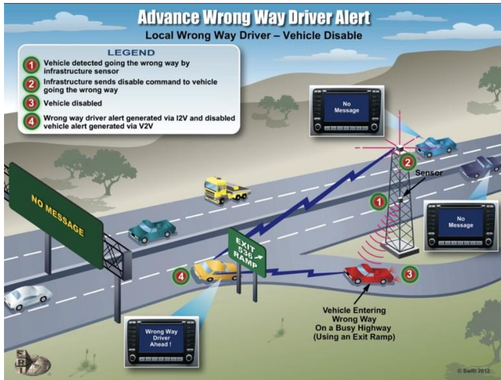
Figure 2-5: Advance Wrong-way Driver Alert – Local Wrong-way Driver in Disabled Vehicle (Randolph, 2014)
