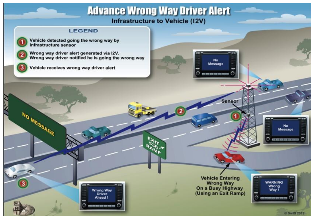
Figure 2-2: Advance Wrong-way Driver Alert – Infrastructure to Vehicle (Randolph, 2014)
