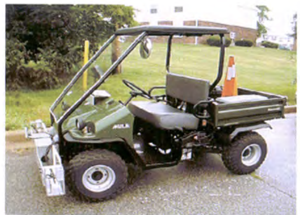
Figure 4. Lightweight profiler (Swanlund 2000).
