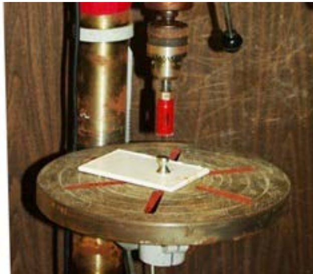
Figure 9. Photo. Drill press to score a test area around a dolly.
