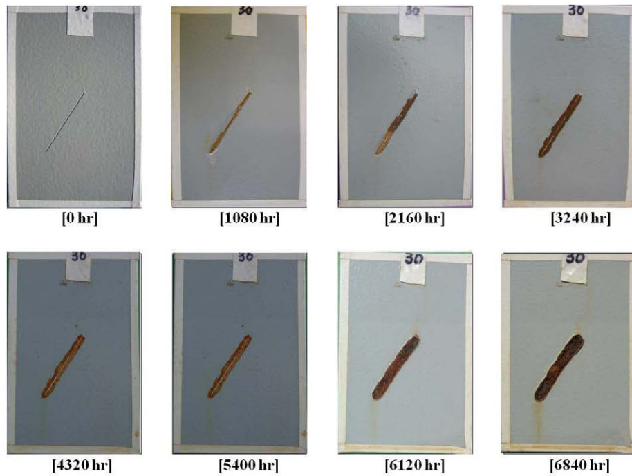
Figure 23. Photo. Progressive changes of panel 30 (two-coat: ALT).
