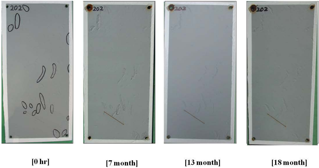
Figure 46. Photo. Progressive changes of panel 202 (WBEP: NW).
