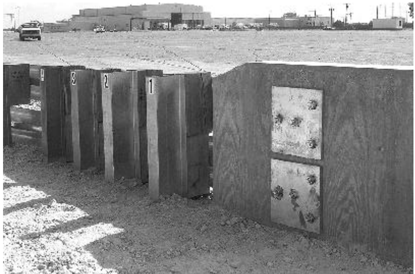
Figure 20. Vertical wall transition prior to test 404211-2.
