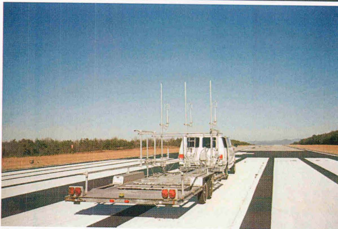
Figure 4.1 Van and trailer configuration for wake turbulence study. Top picture depicts the trailer/sonic setup; bottom picture shows view facing NE.
