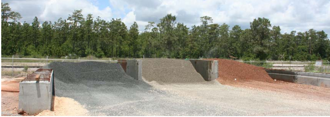
Figure 3. Photo. Lightweight aggregate stockpiles at precaster's facility with continuous sprinklers.
