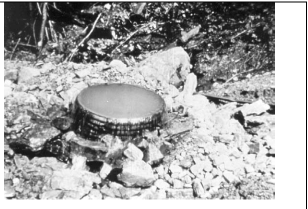
Figure 53b. COE stilling well.
