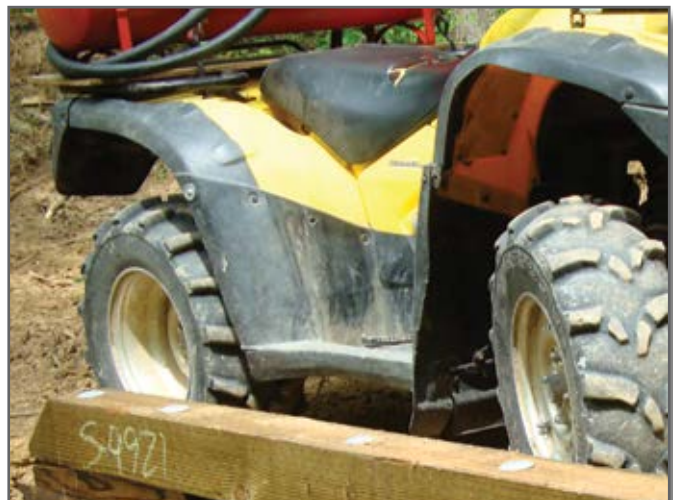
Figure 7—The curbs are difficult to drive over with all-terrain vehicle tires without intentional effort. The ends are beveled to protect the tires from abrupt impacts.
