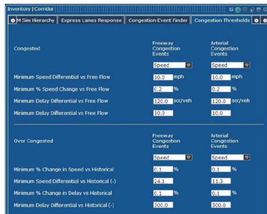
Figure 5: Snapshot of system operator interface for specifying congestion threshold (Source: Dion and Skabardonis, 2015)
