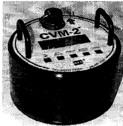
Figure 224. CVM-2 continuous vibration monitor. (OZA Inspections)
