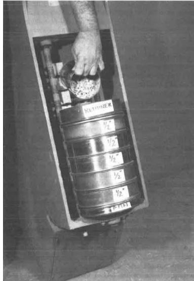
Figure 2-4 Mary Ann sieve shaker used for Pennsylvania Aggregate Retention Test ( source: Kandhal and Motter 1991)
