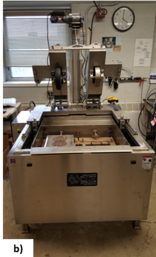
Figure 4-14 HWT device a) before modification (image from Jamescoxandsons.com) and b) after modification.
