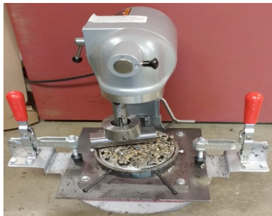
Figure 2-6 Sweep test setup
