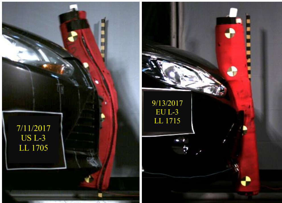
Figure 16. High speed video screen capture of the Flex-PLI at maximum bending at impact location L-3 for the 2012 U.S. (left) and E.U. (right) Ford Focus. The U.S. Focus produces greater bending than the E.U. Focus.
