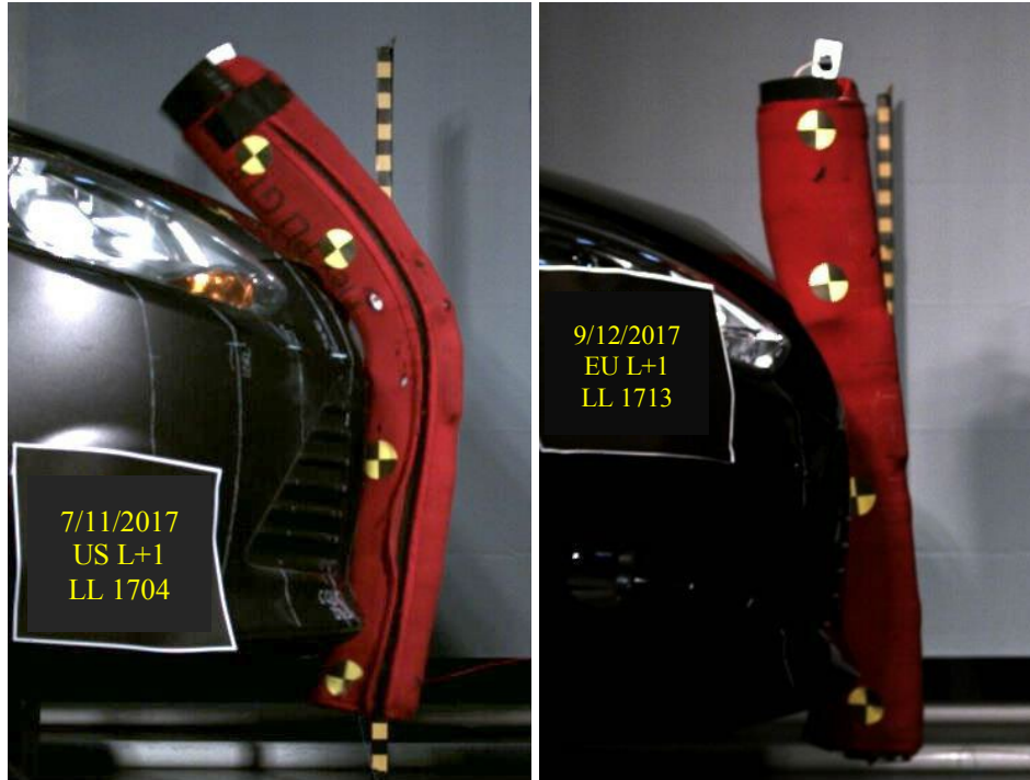
Figure 15. High speed video screen capture of the Flex-PLI at maximum bending at impact location L+1 for the 2012 U.S. (left) and E.U. (right) Ford Focus. The U.S. Focus produces greater bending than the E.U. Focus.
