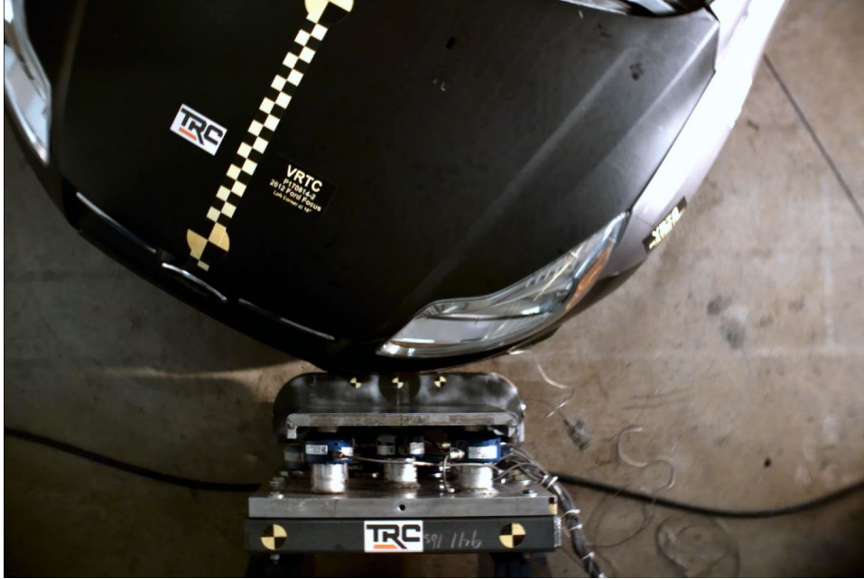
Figure 9. Front bumper corner impact. Pendulum contact with the absorbers is present in both the U.S. and E.U. Focus.
