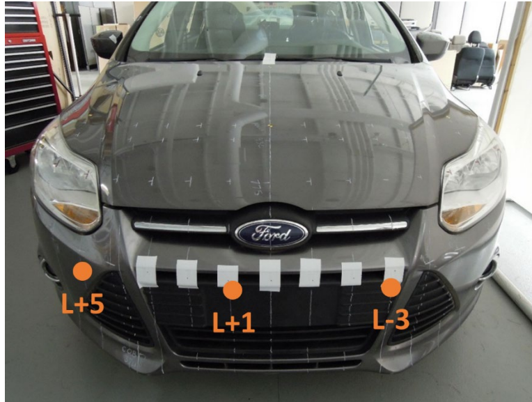
Figure 11. Lower legform impact points for the 2012 U.S. and E.U. Ford Focus
