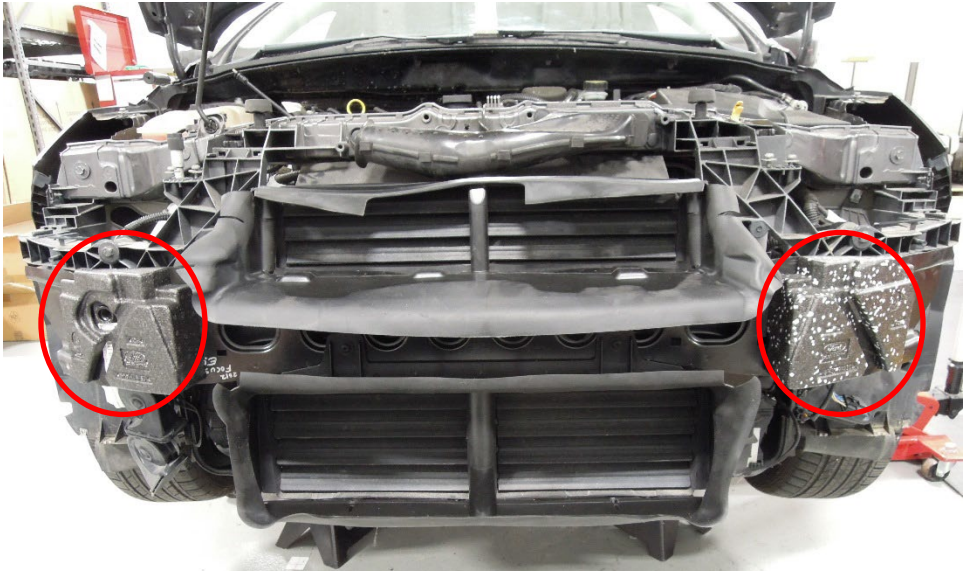
Figure 5. 2012 E.U. Ford Focus front bumper absorber configuration. The bumper absorbers (red) only cover the bumper beam support areas with empty space along the middle of the bumper.
