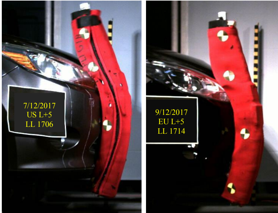
Figure 17. High speed video screen capture of the Flex-PLI at maximum bending at impact location L+5 for the 2012 U.S. (left) and E.U. (right) Ford Focus. Both U.S. and E.U. versions of the Focus produce similar bending.
