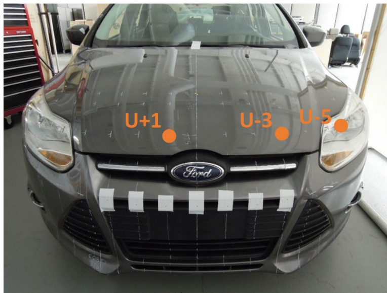
Figure 18. Lower legform impact points for the 2012 U.S. and E.U. Ford Focus
