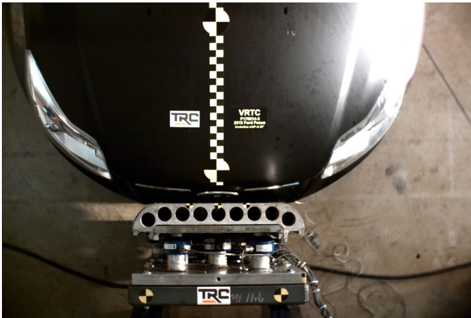
Figure 10. Front bumper impact at centerline. For the E.U. Focus, pendulum contact lies between the absorbers. Pendulum contact is present in the U.S. Focus.
