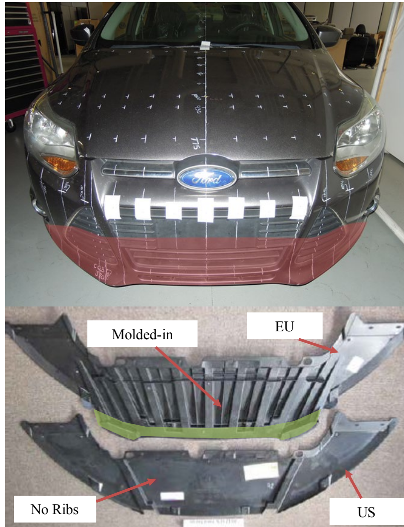
Figure 6. Top image shows the location (highlighted in red) of the underbody deflector panels. Bottom image shows the differences between the 2012 U.S. and E.U. Ford Focus underbody deflector panels. The additional material in the E.U. deflector is highlighted in green
