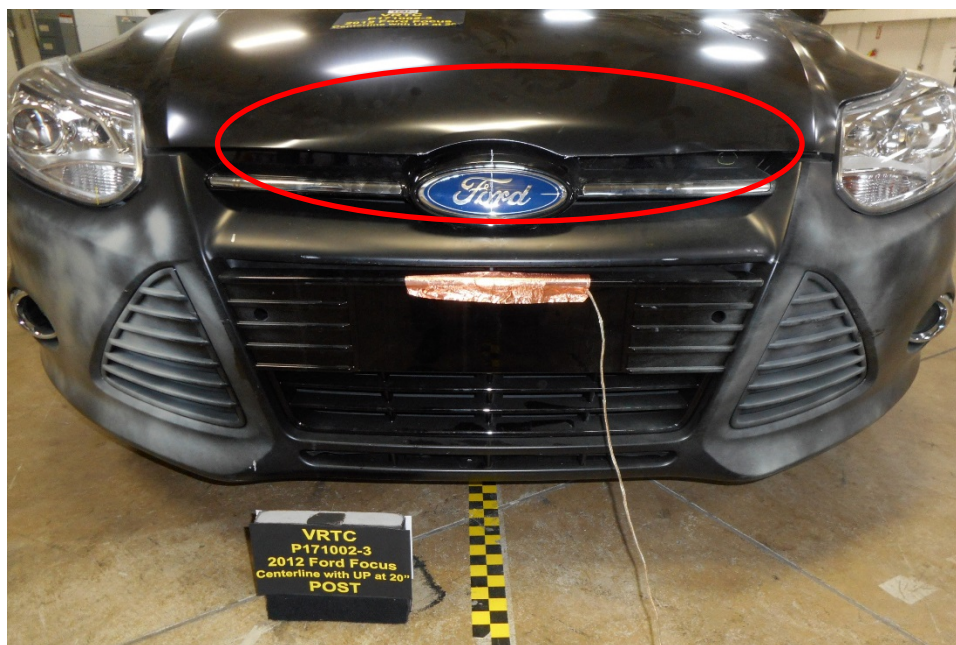
Figure 29. Hood damage (crumpled/bent hood leading edge) to the E.U. Ford Focus (circled in red) that was not observed in the U.S. Focus.
