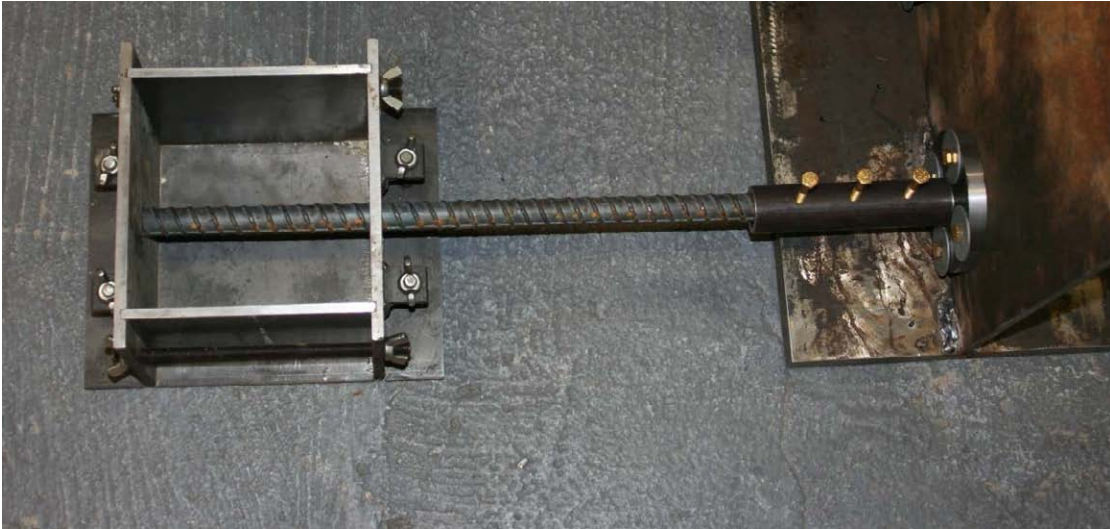
Figure 17. Photograph. Setup for casting pullout specimens.
