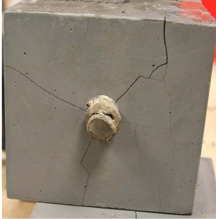
Figure 9. Photograph. End view of a specimen made with material T1 at demolding.
