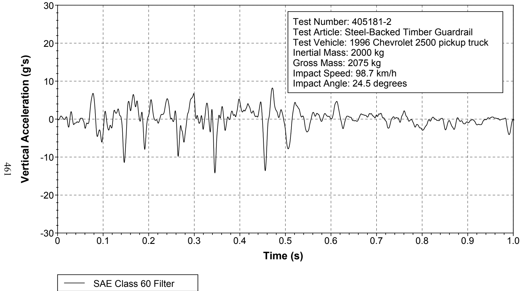
Figure 242. Vehicle vertical accelerometer trace for test 405181-2 (accelerometer located over rear axle).
