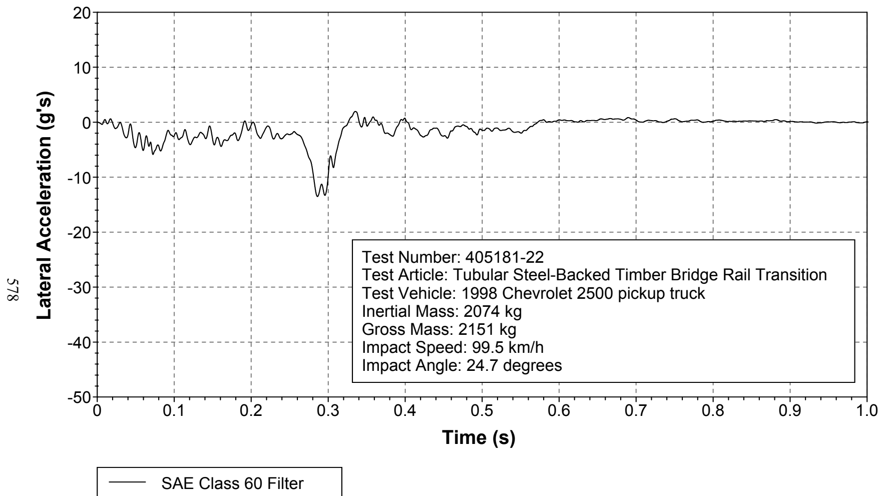
Figure 359. Vehicle lateral accelerometer trace for test 405181-22 (accelerometer located over rear axle).
