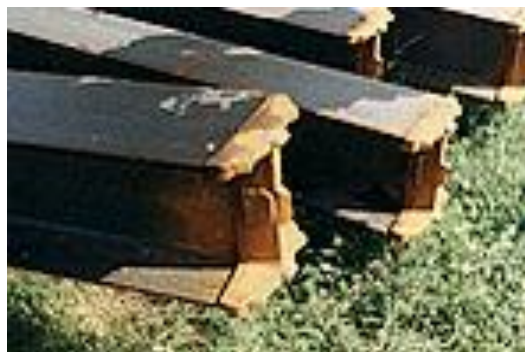
Figure 5 Example of pile tips.
