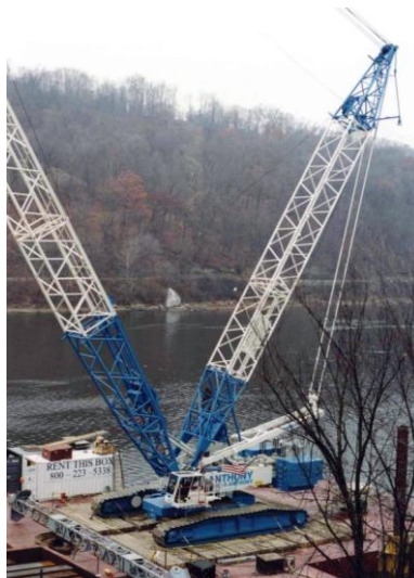
Figure 3 Photograph of a lattice boom crawler crane
