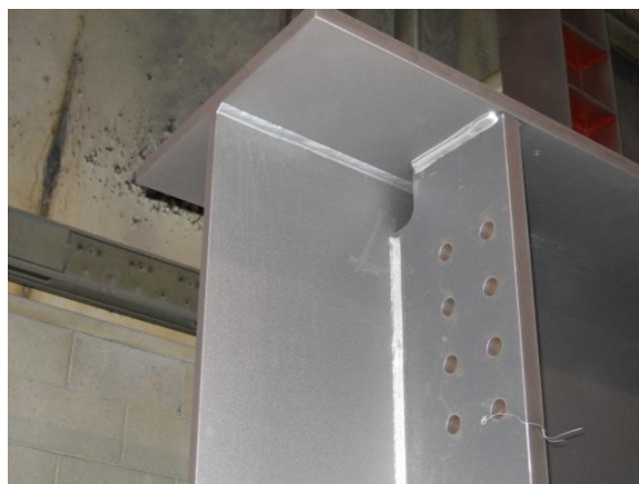
Figure 17 Photo showing a girder after blast cleaning
