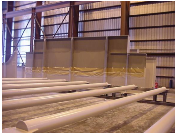
Figure 18 Photo showing painted members in a fabrication shop, note the masked area is for prime coat only
