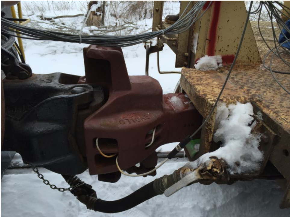
Figure 2-11. Dynamometer coupler installed in Test Car 1 (right)
