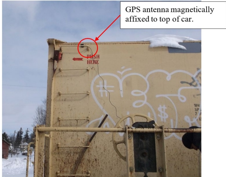
Figure 2-3. GPS antenna installed on Test Car #1
